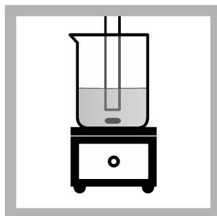
7. Put the probe in the solution. Do not let the probe touch the stir bar, bottom or sides of the container. Remove the air bubbles from under the probe tip.
