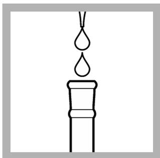
1. Use a pipet to add 5 mL of Nitrate ISA Solution into a plastic 100-mL volumetric flask.
