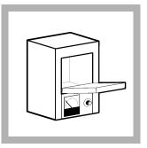
**10.** Put the aluminum dish into a pre-heated muffle furnace at 550 °C (1022 °F) for 30 minutes.
