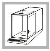
9. Use an analytical balance to weigh the dish to the nearest 0.1 mg (0.0001 g). Record this mg value as A.
