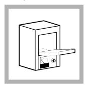
1. Put an aluminum dish in a drying oven at 550 °C (1022 °F) for 1 hour.
