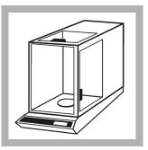
**12.** Use an analytical balance to weigh the dish to the nearest 0.1 mg (0.0001 g). Do steps 10–11 again, until the difference between two successive sample weighings is not more than 4% or 0.5 mg, whichever is less. Record this mg value as B.
