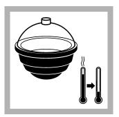
8. Remove the dish from the oven. Let the dish temperature decrease to room temperature in a desiccator.
