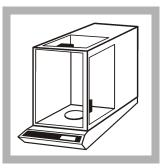
**4.** Use an analytical balance to weigh the dish to the nearest 0.1 mg (0.0001 g). Record this mg value as C.
