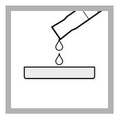
**5.** Mix the sample. Add 50 mL of the sample to the aluminum dish.
