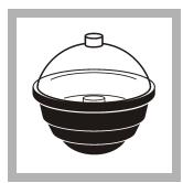
**11.** After 30 minutes, remove the dish from the furnace with tongs. Let the dish temperature decrease to room temperature in a desiccator.
