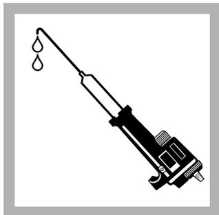
2. Hold the Digital Titrator with the cartridge tip up. Turn the delivery knob to eject air and a few drops of titrant. Reset the counter to zero and clean the tip.
