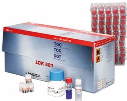
*Cuvette test for TOC determination by the difference method*
