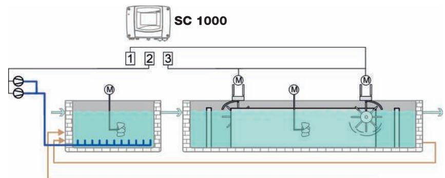
Fig. 3: Diagram of the plant and the SC 1000 relay connections
