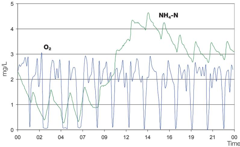
Fig. 4: Typical time-course curve of the 2 point control in the oxidation ditch.
