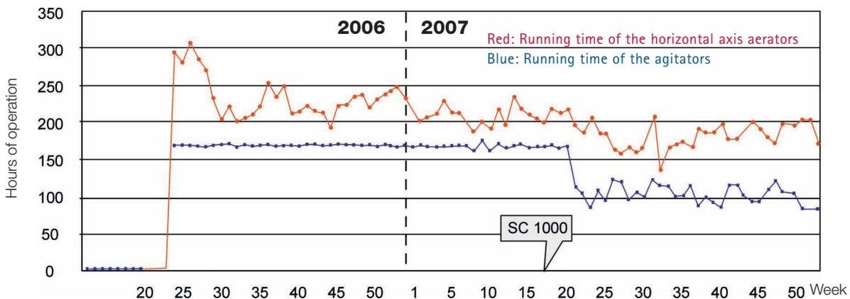
Fig. 5: From week 17/2007, the SC 1000 controller reduced the run time of the horizontal axis aerators and agitators in the oxidation ditch by up to 20 %.
