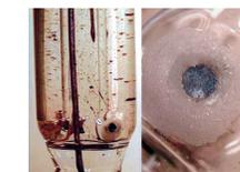
Ceramic diaphragm blocked by a sulphide deposit
