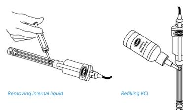
Removing internal liquid
